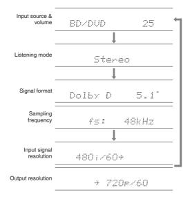
If "Dolby D 5.1" is displayed in signal format, the Dolby Digital 5.1 ch signals are being input. When listening to AM/FM radio, the band, frequency and preset number are displayed.
